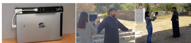
Figure 2. 3D reconstruction of the priest of the Asinou church (middle, right) using the occipital structure sensor (left)
