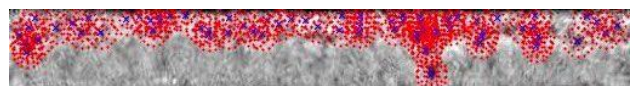
Figure 9. Iris image key points (blue) and points around them (red) used to calculate key points descriptors
