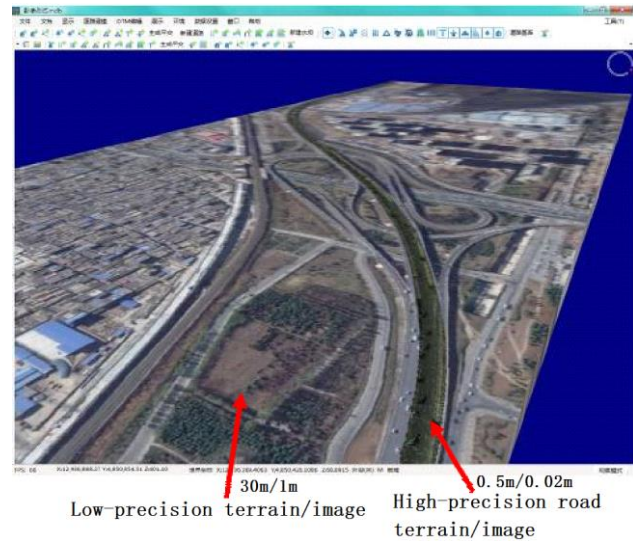
Figure 3 Schematic diagram of fusion and 3D application of high and low precision data
