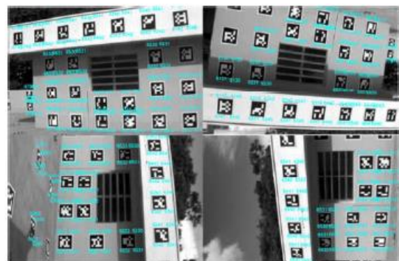
Figure 2. Examples of hyperspectral images used in the camera calibration.
