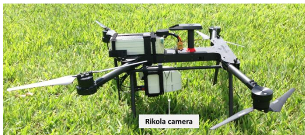
Figure 3. UAV platform with the Rikola hyperspectral camera.
