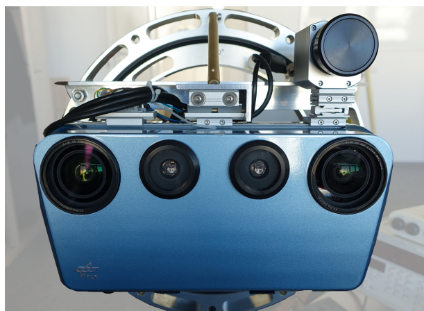
Figure 1. IPS Camera System with Optris PI 450 attached on top. The system is mounted on a rotary plate for calibration purposes.
