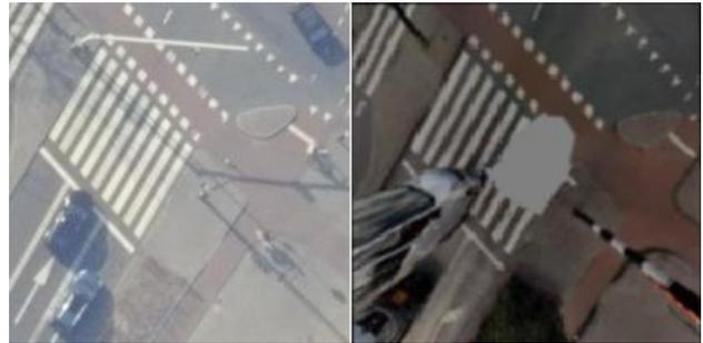
Figure 1. Left: Aerial nadir image, right: re-projected MM image
