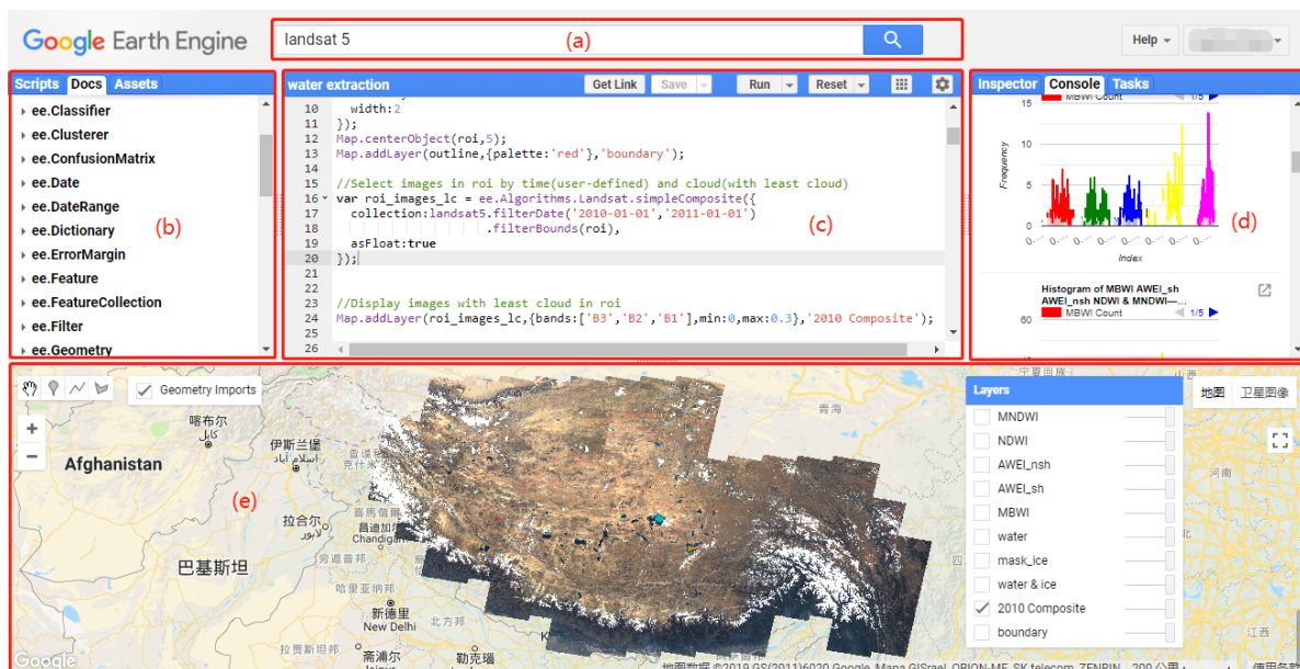
Figure 2. The interface of GEE: (a) is for data retrieval; (b) is for code preservation, document query and resource uploading; (c) is for code editing; (d) is for information query, result outputting, task downloading and running resource displaying; (e) is for layer displaying
