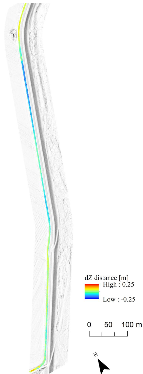
Fig. 4. Visualisation of height differences between the oriented ULS and DIM point clouds overlaying the hillshade model of Tarnobrzeg test sites.
