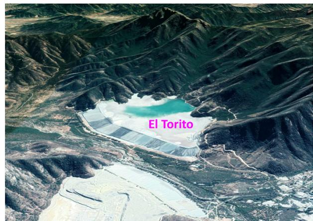
Figure 2. Tailing dam El Torito in Chile
