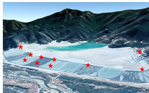
Figure 6. Planned positions (red asterisks) of 10 GNSS devices. 5 corner reflectors will be integrated to five of these positions (under discussion).
