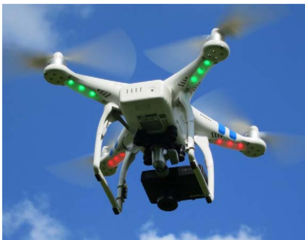
Figure 2. DJI Phantom 2 with mounted Canon Powershot 110 (Bareth et al. 2015)
