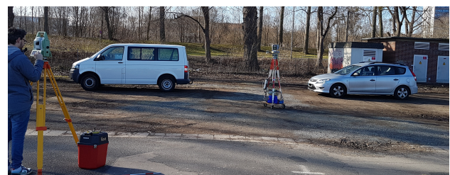
Figure 2. The setting for the measurements: the total station (left), both cars (in the back) and the scanners at the dynamic rack (center)
