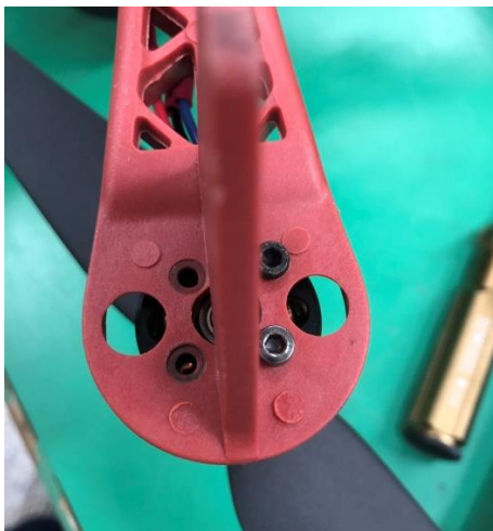
Figure 3. Motor mount asymmetrically loose
