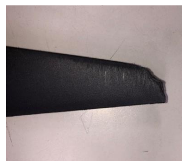
Figure 8. Little damage on the edge of propeller
