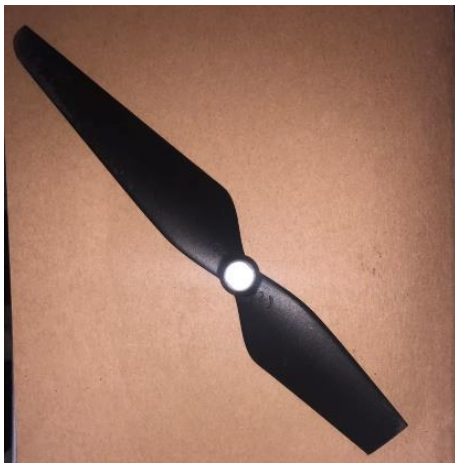
Figure 2. Unbalance broken propeller
