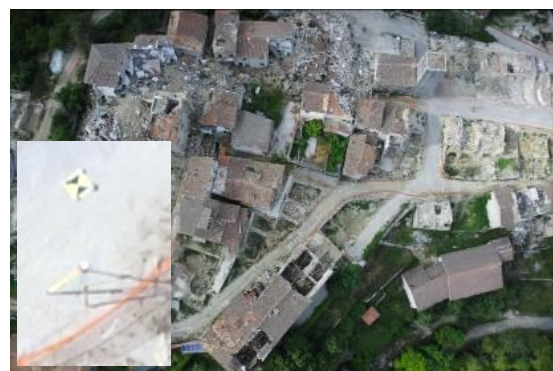
Figure 4. Example of raw image and related level of detail (bottom left, artificial 0.4 x 0.4 m 2 marker and GNSS receiving station mounted on a tripod)
