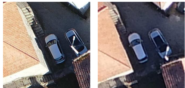
Figure 1. Examples of images acquired from 100 m height, with GSD 3 cm (left) and from 300 m, with GSD 9 cm (right).
