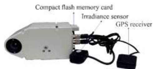
Figure 1. Hyperspectral camera based on a Piezoactuated FPI
