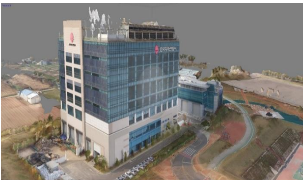
Figure 4 The 3D model generated by combining oblique and Nadir images.
