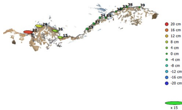
Figure 4. The ChPs error estimation after registration with a) 3 CPs clustered on the north, b) 3 CPs clustered on the south, c) 3 CPs clustered on the middle, d) 3 CPs uniform, e) 8 CPs uniform. The figures have the same ordinary ChPs as the name of 22,24,26,15,11,33,34,35,37 from south to north (left to right)
