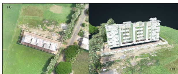
Figure 7: Building outputs generated after data processing (a) Orthomosaic image (b) 3D Building model
