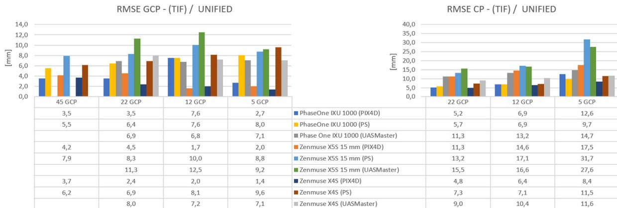
Figure 10. Comparison of the 3D RMSE values at GCPs (left) and CPs (right) as results of the bundle block adjustments with Pix4Dmapper, Agisoft PhotoScan and Inpho UASMaster. Note scaling.
