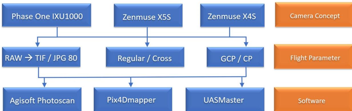
Figure 5. Parameters influencing the geometric quality of the image blocks
