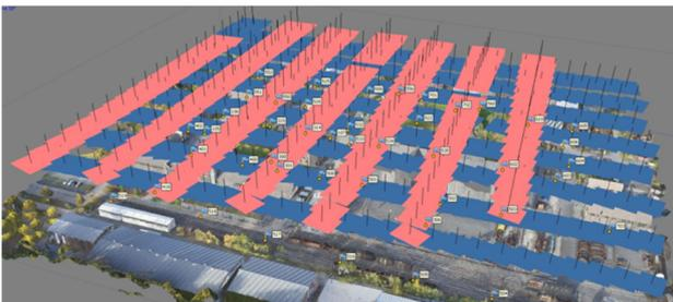
Figure 4. Flight arrangement Regular (R) and Cross (C), (Image block with Zenmuse X4S)
