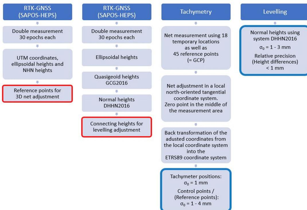
Figure 3. Workflow of geodetic measurements and data processing (GCG2016 - German Combined QuasiGeoid, the height reference for the transition between geometric heights in ETRS89/DREF91 and physical heights in DHHN2016, the German height reference system).
