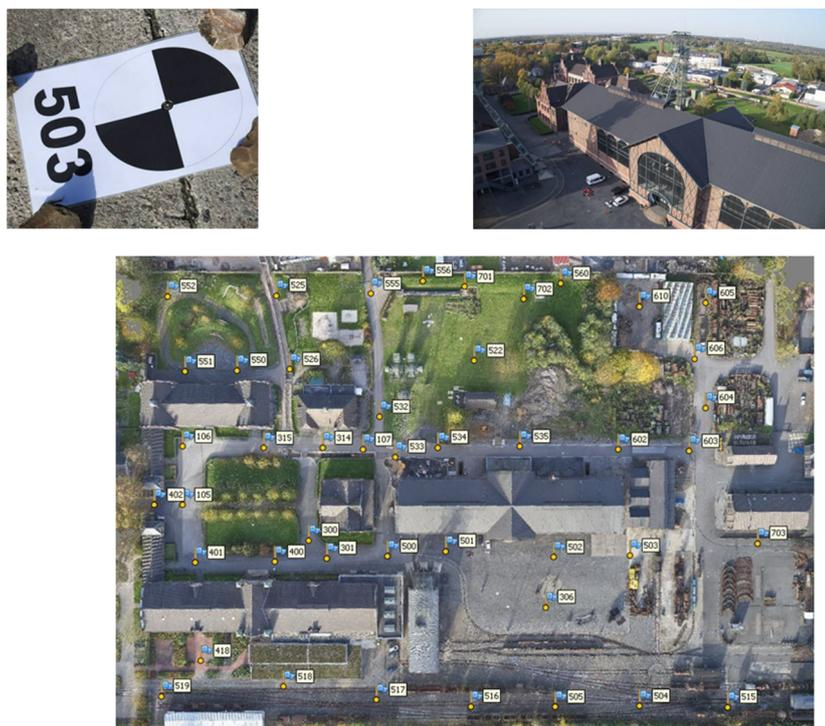
Figure 2. UAV test field Zollern colliery. Top: Target for signaling the GCPs and the view of the area. Bottom: Point cloud with signaled GCPs (UAV flight from October 2017)
