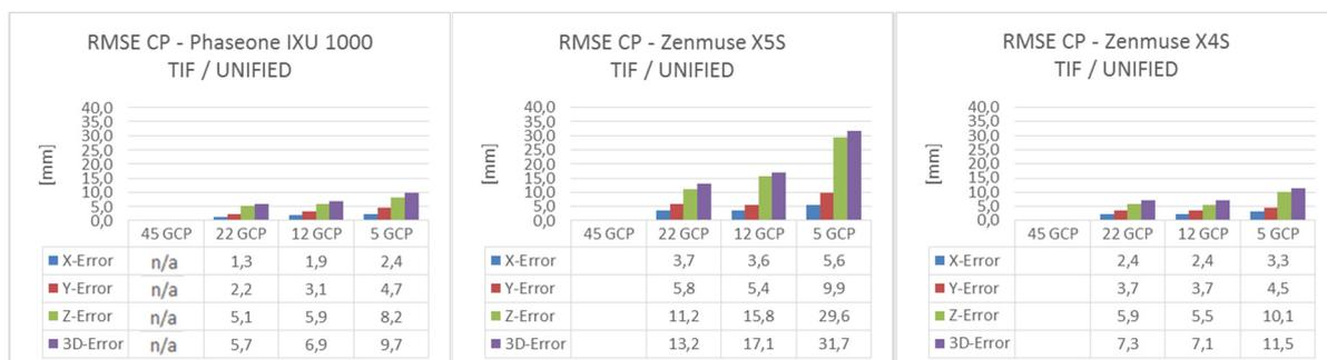
Figure 7. RMSE values at CPs. Flight arrangement: RC. ONE set of interior orientation parameters (UNIFIED). Calculation: Agisoft PhotoScan
