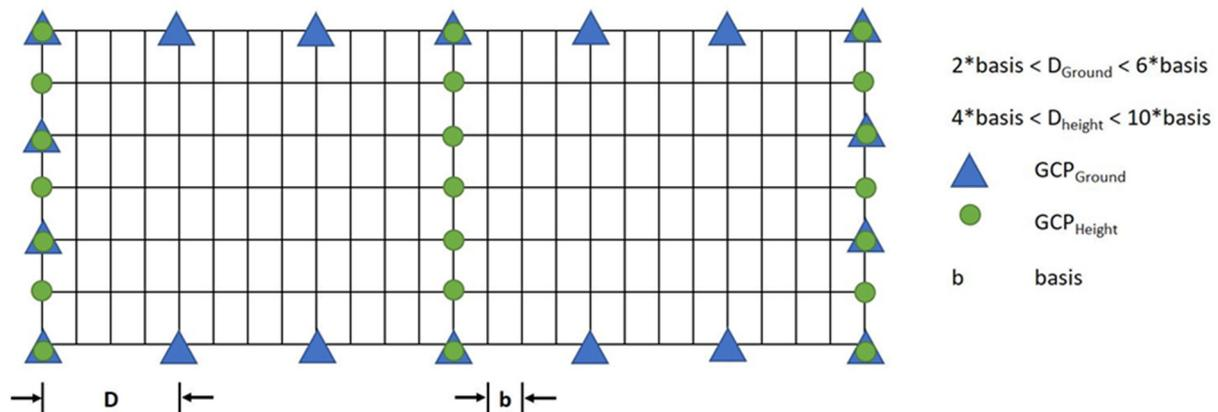
Figure 6. Schematic arrangement of GCPs during (analogue) image flight (Kraus 1994)
