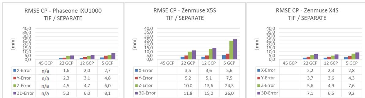
Figure 8. RMSE values at CPs. Flight arrangement: R+C. TWO sets of interior orientation parameters (SEPARATE). Calculation: Agisoft PhotoScan.
