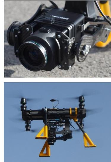
Figure 2. Phase One IXU 1000 (100Mpix) (top), Coptersystems Multicopter (bottom)
