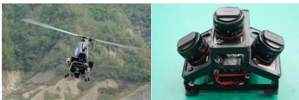
Figure 2. The adopted unmanned helicopter and three-camera imaging system.
