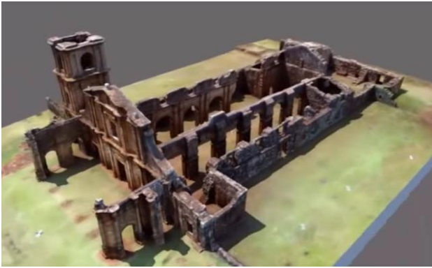
Figure 12. Fusion of 3D models produced by Photogrammetry and TLS (Reiss et al, 2016).
