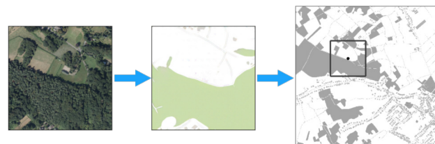
Figure 1. Method Overview: First, an aerial image is collected, then it is segmented into a map-like representation, finally it is matched within a reference map for localization of the vehicle.
