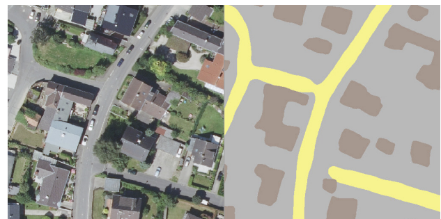
Figure 4. On the left aerial image that serves as input to the image segmenter. On the right segmented image. Building footprints in brown and roads in yellow.
