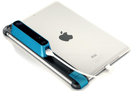
Figure 2: Occipital Structure Sensor attached to an iPad. Image taken from (Hoffman, 2014).
