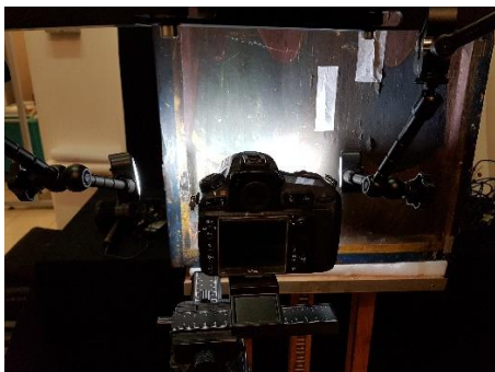
Figure 2. Macro shooting lights and camera setup
