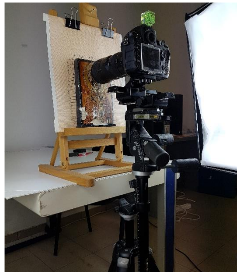
Figure 4. Setup for macro shooting. Vertical graded slider and horizontal X-Y graded slider.
