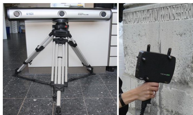
Figure 3. Steinbichler T-Scan 2: Optotrak Tracking system and handheld laser scanner. (Rahrig/Drewello 2012)
