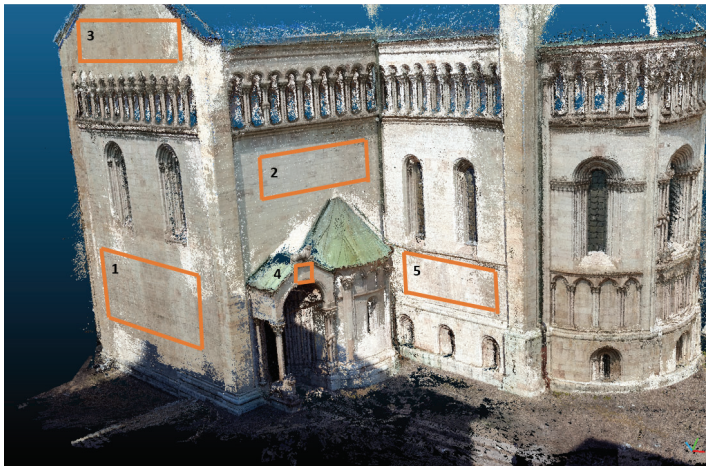
Figure 4. Locations of the five areas used to calculate the plane fitting RMSE useful to evaluate geometric performances of the video-based 3D reconstruction.
