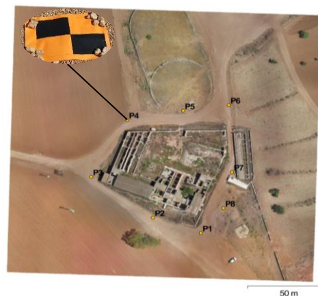
Fig. 4. Distribution of GCPs for the georeferencing of the photogrammetric project, overlapped to orthoimage obtained from photogrammetric project Two flights were made; the first at a height of 50 m above ground level, with an autopilot using the DJI GS Pro © application to obtain nadiral photographs. The flight plan consisted of 11
