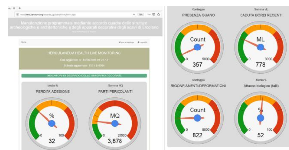
Figure 6: Gauge charts (created with Google Charts - https://developers.google.com/chart/interactive/docs/gallery/gauge ) used to visualize dynamic data to monitor the state of decay of the site.
