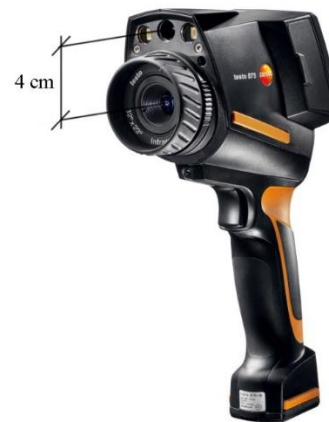
Figure 6. Thermal camera with distance between IR and RGB sensors
