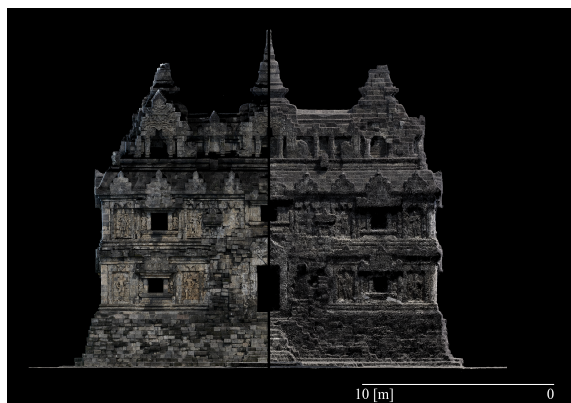
Figure 4. Orthoview of the Candi Sari point cloud from both laser scanning (left) and image matching of drone images (right)
