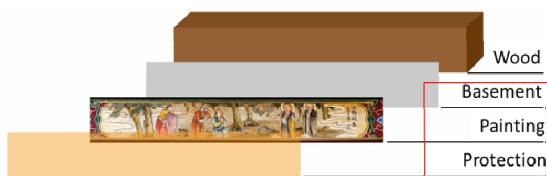
Figure 3. Different layer of the painting on the wood
