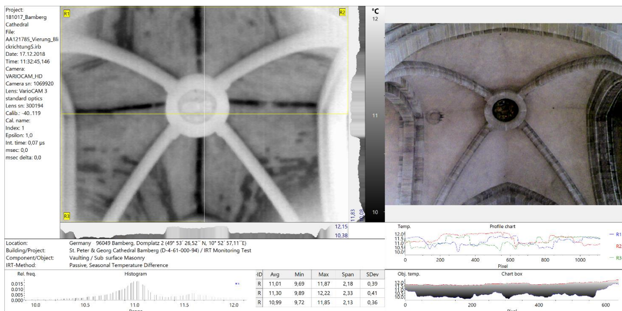
Figure 5: Greyscale visualisation and radiometric measurements of the vaulting structure over crossing of transept and aisle, depicting masonry construction, variations in fabric, stone sizes and pattern.
