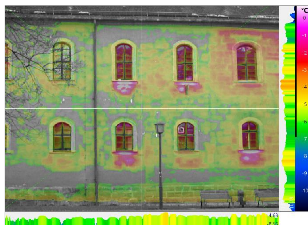
Figure 3: Merging of thermal and visual image. Location of the extent and position of the radiometric data.
