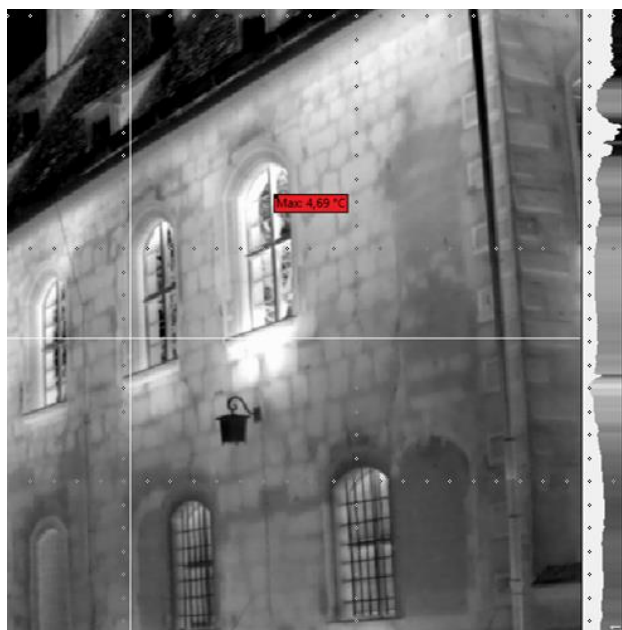
Figure 4: Greyscale visualisation of subsequently walled up openings under plaster.
