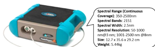
Figure 2. Picture and parameters of ASD FieldSpec4 portable spectroradiometer
