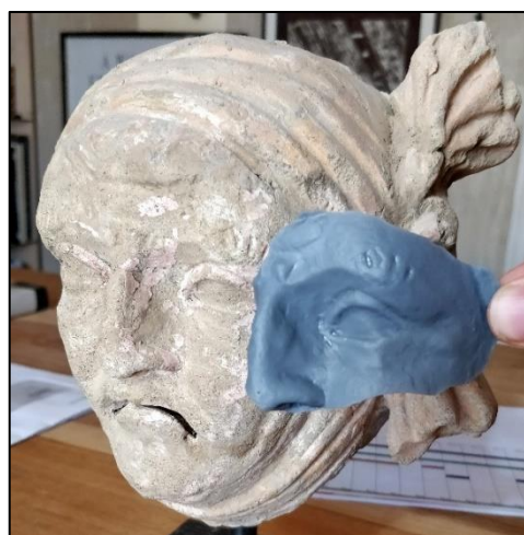
Figure 14. 3D printed segment compared to original
