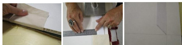
Figure 19 - Three moments of applying the Velcro strips on the back of the panels.
