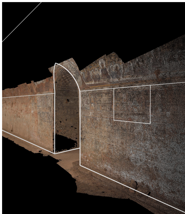
Figure 12. Photogrammetry point cloud in BIM of west wall painting.
