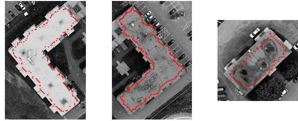
Figure 3. 3D building boundary points projected onto the optical image, i.e. \mathbf{TB}_i , which are used to initialize the snake model and for the energy term E_{ShapeSim} .
