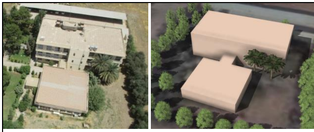
Figure 9. Left: UAV image captured from inclined view; right: image of same building produced from free satellite imagery, without textures and missing details
