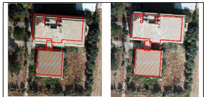
Figure 4. Processed stereo imagery showing the digitised boundary, with the building location digitised using photogrammetric software
