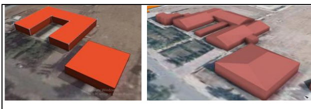
Figure 10. Two levels of details for the same buildings: (left) LoD1 from satellite imagery, (right) LoD2 from aerial imagery
