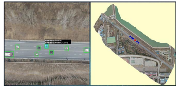
Figure 7. Moving vehicle targets detection and geolocation for different flight altitude. ( In the left figure, the green box is used to express different classes of vehicle targets detected by the YOLOv3 network model. The pixel coordinates of the vehicle detected center point are indicated by red crosses, and the blue box shows the geo-location of the target, the red box shows the selected target in the right figure on the reference map. )
