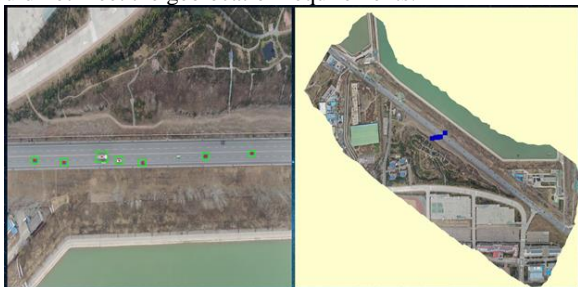
Figure 9. flight altitude 300m vehicle detection and geolocation
