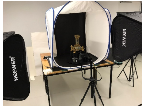
Figure 5. Natural light acquisition setup. Objects are placed in tents and flashed are mounted with snoods.
