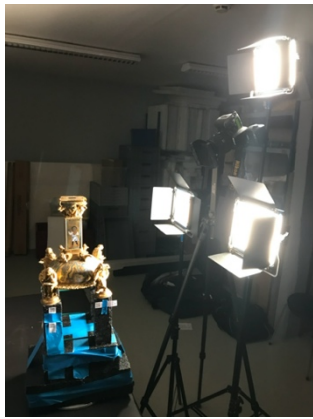
Figure 7. Setup for acquisition in cross-polarised lighting condition. A linear polarizing filter is placed in front of the led panels. A rotative linear filter is mounted on the lens in order to active or inactivate the polarization.
