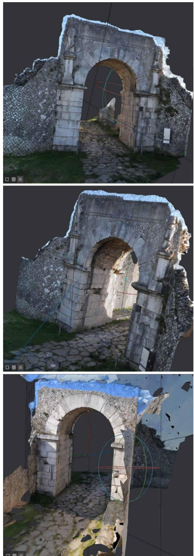
Figure 9. definitive 3d model with texture from Meshroom.
