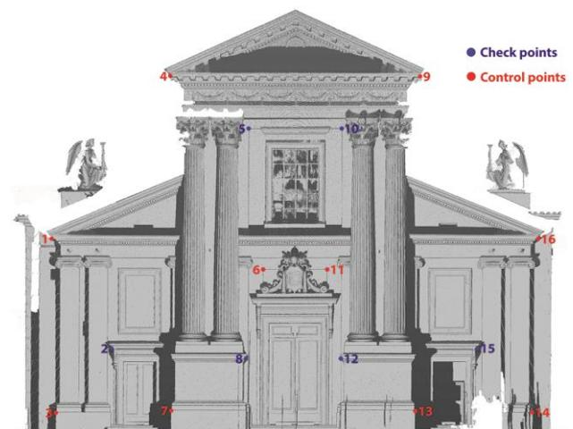
Figure 5. Point cloud from laser scanner with GCPs.
