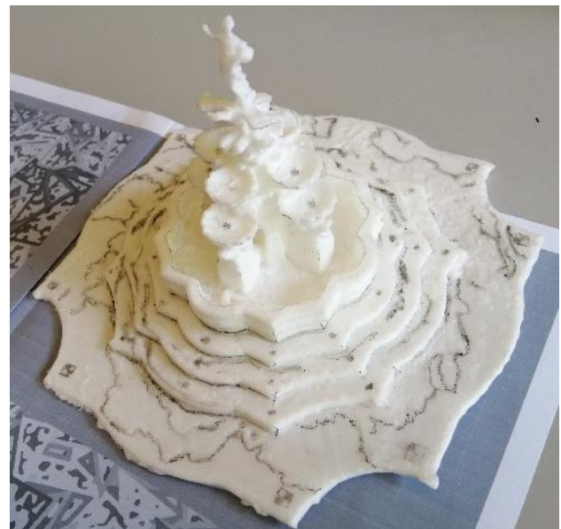
Figure 8. The 3D printed model of the Garraffo fountain with the targets drawn on the surface.
