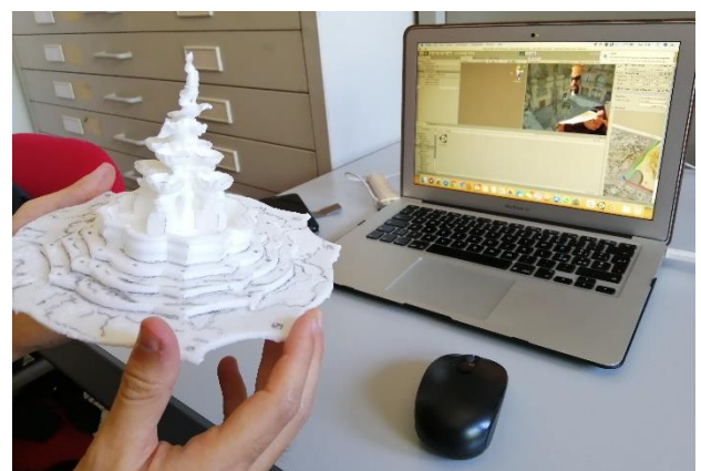
Figure 9. The 3D printed model of the Garraffo fountain with the targets drawn on the surface.
