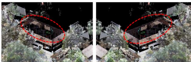
Figure 1. Incomplete building's pointclouds on the roof part (denoted by red circle) as the result of Terrestrial Lidar acquisition.
