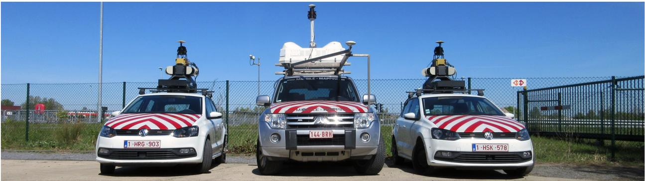
Figure 1. Example Mobile Mapping Systems: IP-S2 Compact system (left and right) and Lynx mobile mapper system (centre).
