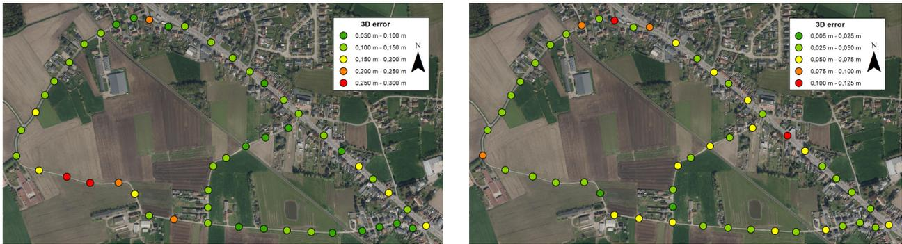
Figure 5. 3D errors of GCP in rural dataset for the low-end system (left) and high-end system (right).
