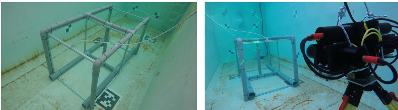
Figure 6. Scanning setup in the test tank. Left: Test structure constructed from aluminum profiles and polypropylene pipes, Right: Underwater laser scanner deployed on a tripod.
