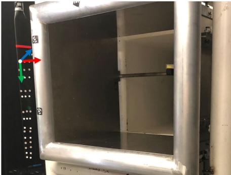
Figure 6. Mounted rotor blade in the wind tunnel; Realisation of the reference coordinate system
