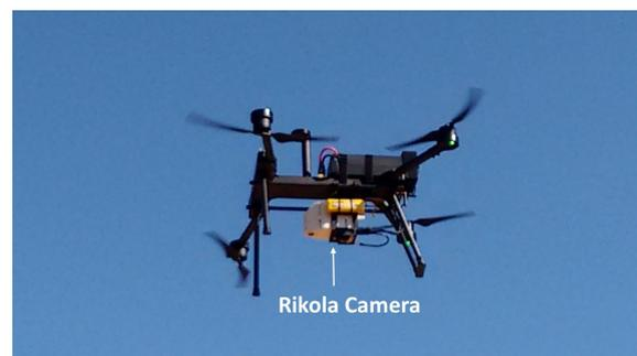
Figure 4. UAV with the FPI camera on board.
