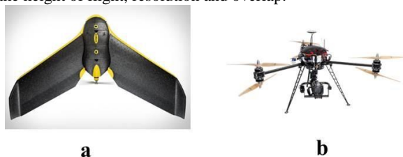
Figure 1: UAVs utilized in the study: (a) Ebee, (b) HDS3.
